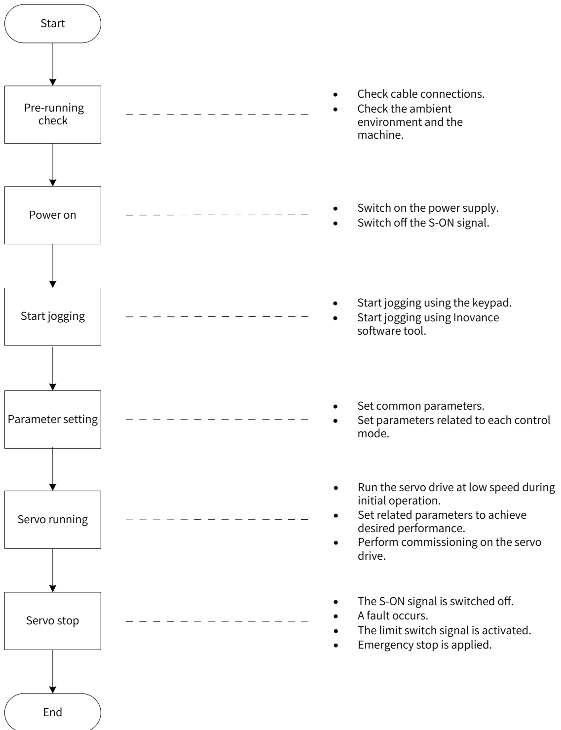
Figure 5-1 Flowchart for setting the servo drive
