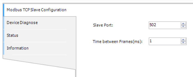
Figure 3-49 Modbus TCP slave configuration
