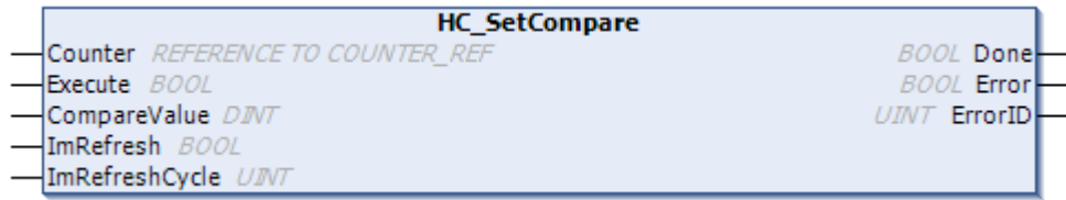
Figure 6-2 Diagram of the HC_SetCompare function block
