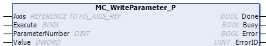
Figure 6-26 Diagram of the MC_WriteParameter_P function block
