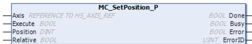
Figure 6-27 Diagram of the MC_SetPosition_P function block
