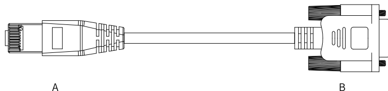
Figure 3-45 Outline drawing of the PC communication cable
